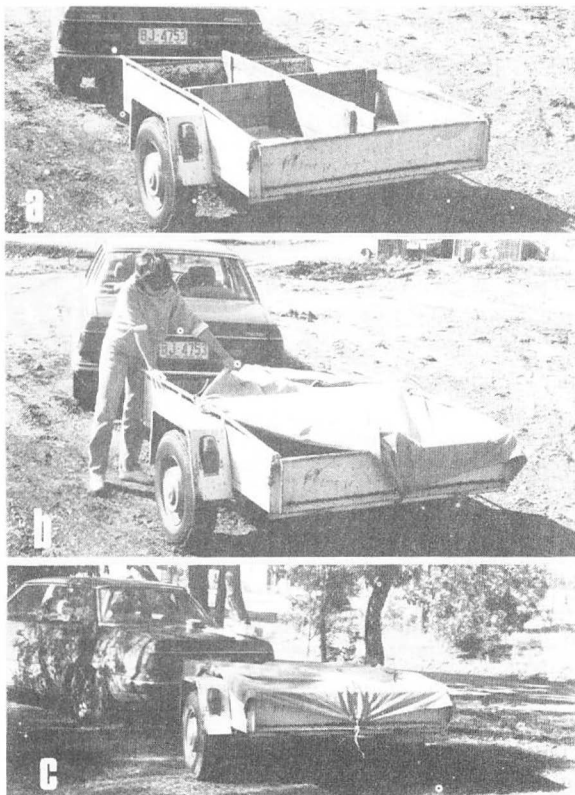
Figure 1. Photographs showing details of operation of holding trailer (a) tarpaulin removed to show the wooden boards which form the four compartments; (b) tarpaulin cover affixed to trailer with corner flaps open; (c) cover trailer under shade for processing of birds.
