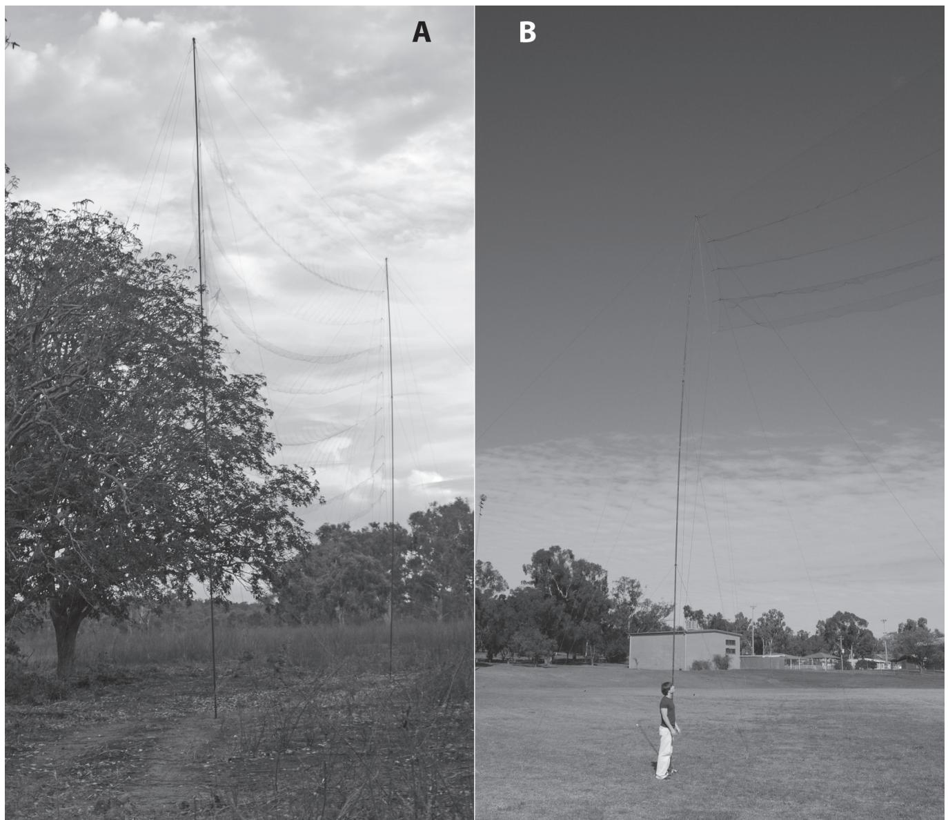
**Figure 5.** 12-metre-high pole set-up with mist nets. A: In situ set-up with two 18-metre-long nets in parallel, next to a mature *Canarium australianum*, Northern Territory. B: Set-up with one net, operator shown for comparison.
