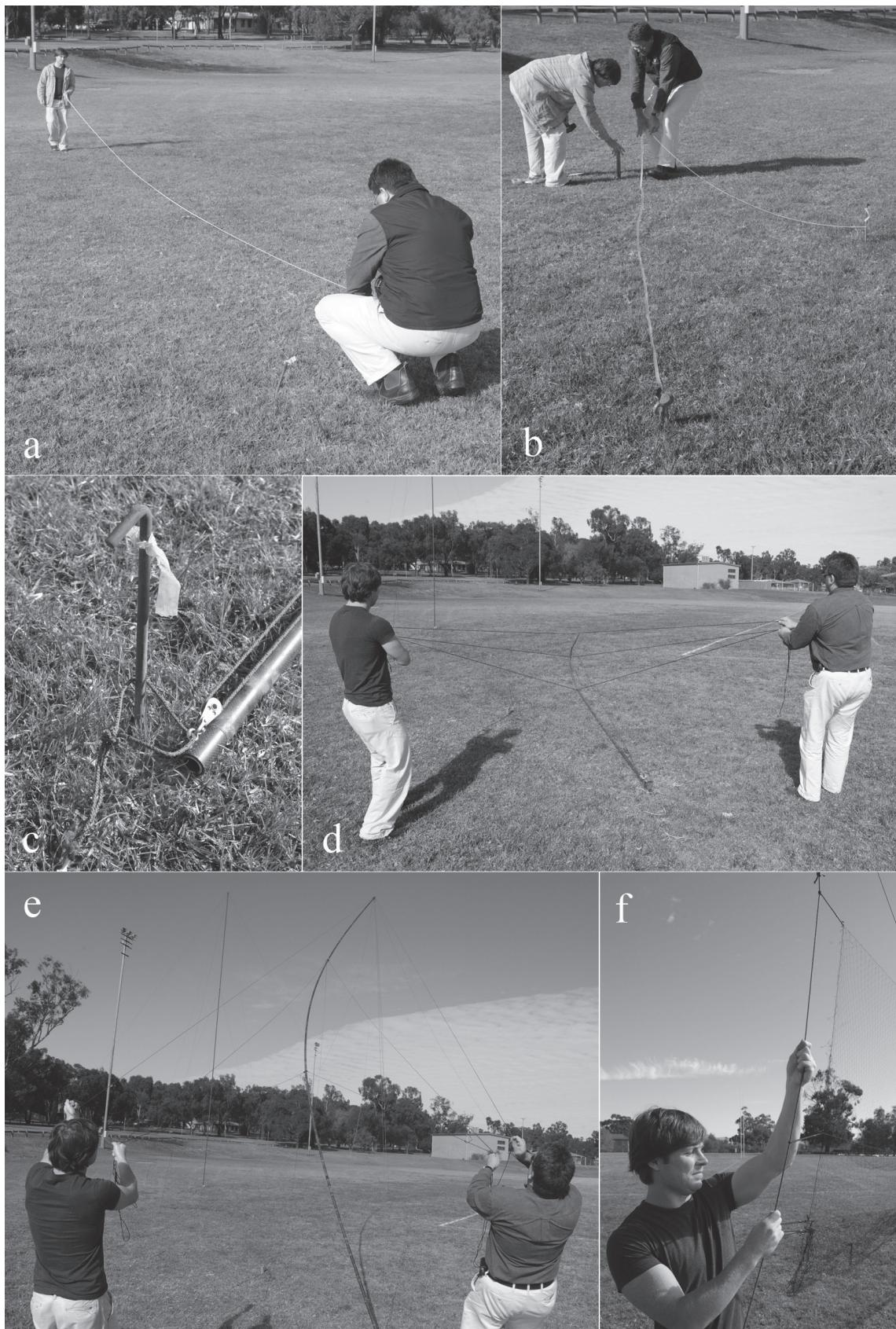
**Figure 4.** Photograph series of pole and net set-up, including: a) measuring out the net line; b) measuring out and placing guy rope pegs; c) attachment of the base of the pole to the peg marking the location of the raised pole; d) operators placing even tension on the guy ropes; e) operators raising the pole in a steady, even motion, and f) raising the 'flagpole' rope and opening out the net at the same time.
