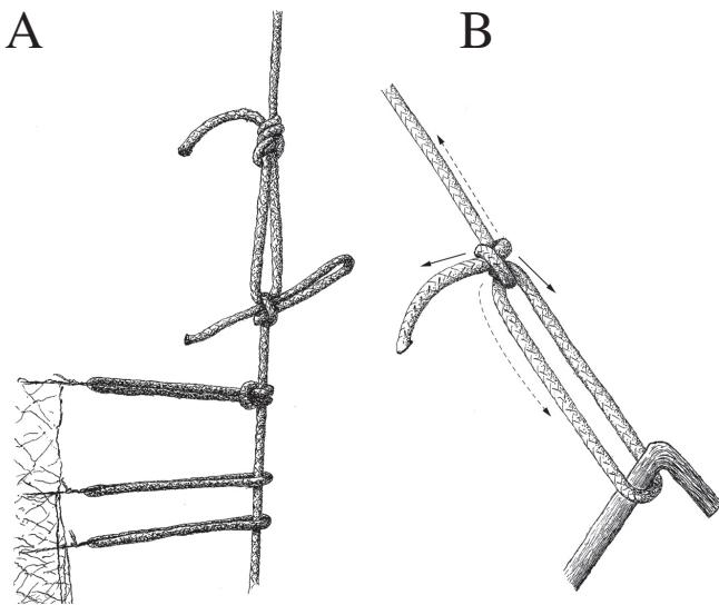
**Figure 3.** **A:** Illustration of part of the 'flagpole' rope; including the upper tail with loop, the lower tail which is tied onto the loop with a half-hitch and the arrangement of net loops on the rope. **B:** Illustration of the lower end of a guy rope with a two half-hitches knot forming a loop running around a peg. This allowed adjustable tensioning of the guy rope (dashed arrows) but must be tightened (solid arrows) to prevent slippage.
