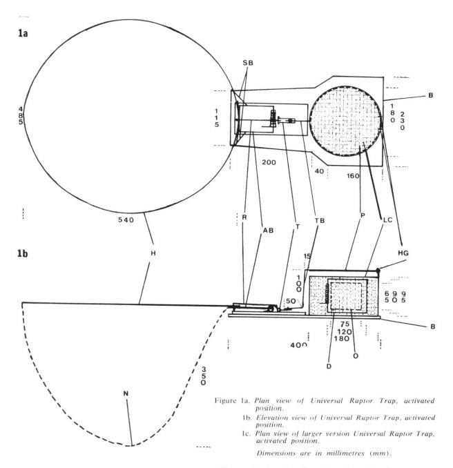
AB = action bar; B = base; D = door; H = hoop; HG = hinge; L = lure; LC = lure cylinder; N = netting; O = door opening; P = platform; R = retainer; SB = stabilizer bar; T = trigger; TB = trigger bar.
