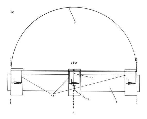
hinges (12-14 gauge). To the opposite side of the platform was soldered a trigger bar (12-14 gauge wire). The wire cylinder was then fastened to the base plate so that the trigger bar rested within the raised lugs of the trigger mechanism.
